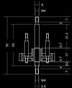
Gear: Aluminium Alloy Shafts: Aluminium Alloy Axle: Titanium Alloy Triangle: Titanium Alloy
