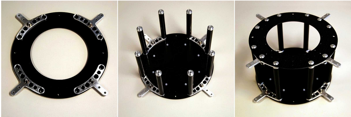
Figure 3.6: Bottom fuselage ring with girder flanges installed (left), with fuselage plate and tubes installed (middle), and complete JAviator V2 fuselage (right).
