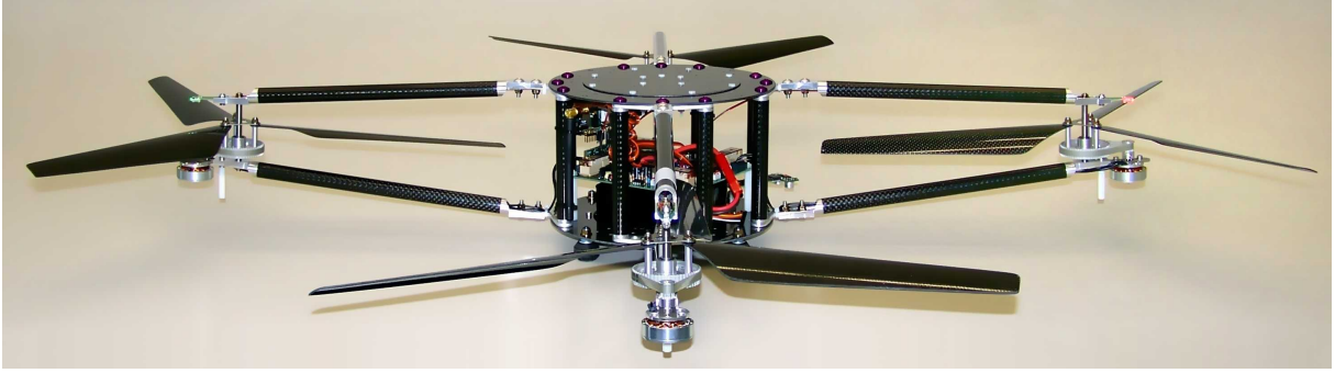
Figure 1.1: The JAviator quadrotor, a high-precision “aerial software testbed”.
