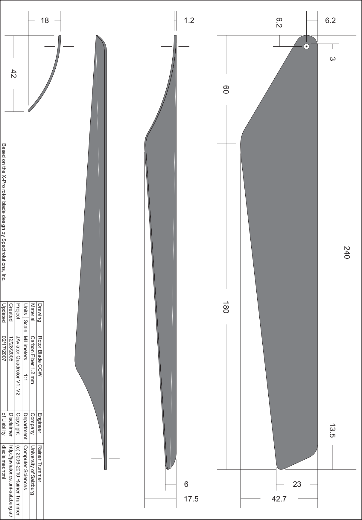
Figure B.16: Rotor blade used to assemble the counter-clockwise spinning rotors.
