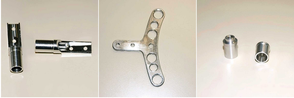
Figure 3.5: JAViator V2 CNC-turned and -milled girder connectors (left), laser-cut girder flange (middle), and CNC-turned fuselage connectors (right).
