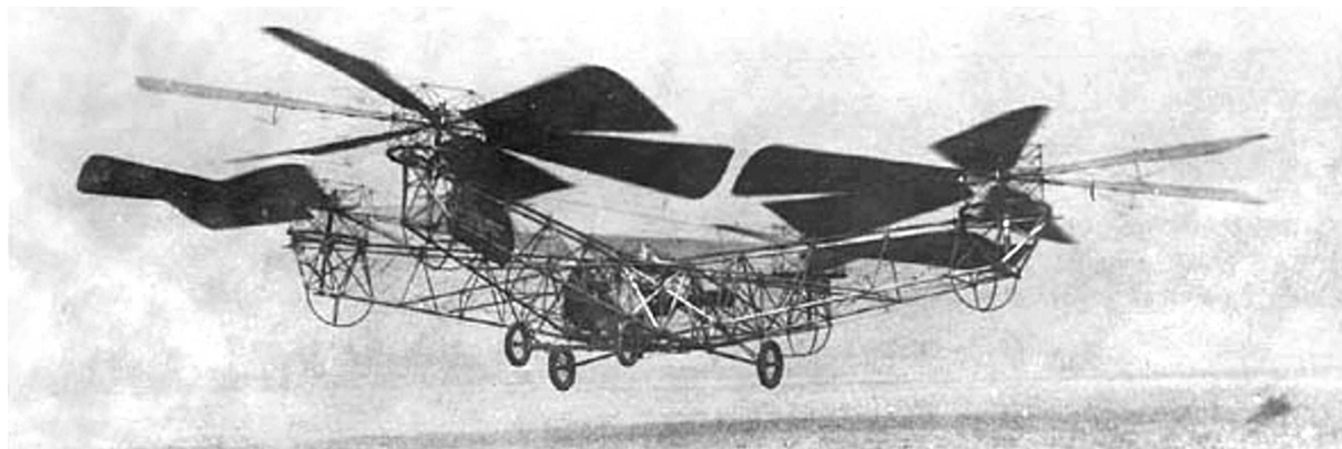
Figure 2.2: The de-Bothezat-Jerome helicopter of 1922 descending after a test flight on February 21, 1923 at McCook Field near Dayton, Ohio. Taken from Edison [50].
