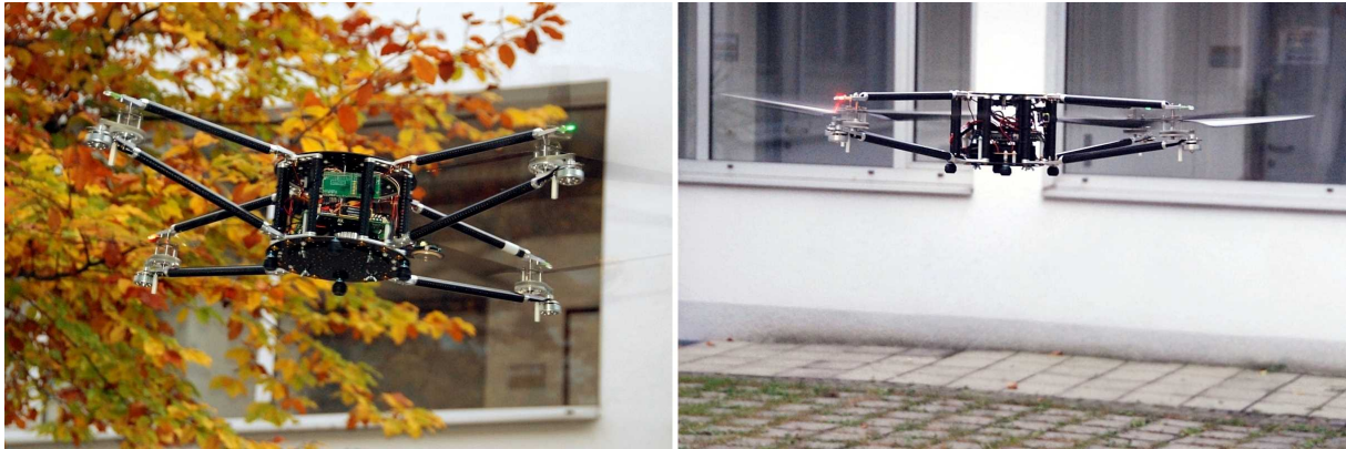
Figure 1.3: Outdoor flights performed in the courtyard of the Department of Computer Sciences at the University of Salzburg, showing the JAviator flying at a height of about 3 m (left) and hovering at a height of about 1.5 m (right).
